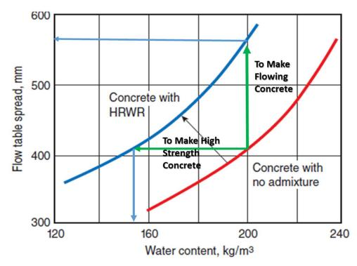
Typical relation between flow table spread and water content of concrete made with and without superplasticizer
